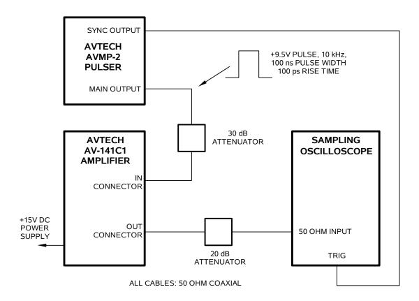
The recommended test set-up is shown above.
